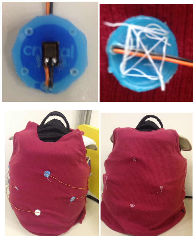
Figure 7. a) Back SG sensor application, b) Front SG sensor application
